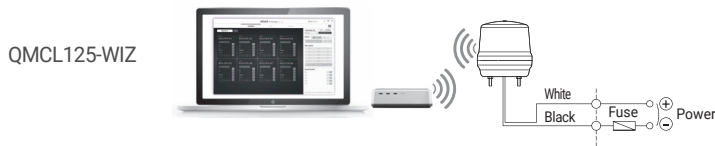
Ethernet connection via Gateway
